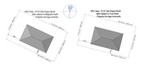
Note that the property lines no longer tag correctly. The QARC Template System provides text labels to overcome this issue. Have a look at *Sheet 102SP - Site Plan 1-200*
